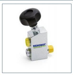
direction and leave the flow in the other direction completely open. This is useable when a controlled return of a cylinder is desired, but when a rapid raise of the cylinder is desired during pumping. VAB114 is mounted directly onto the hydraulic unit via G1/4" thread.
