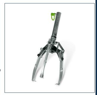
The smaller sizes, 5 ton and 10 ton, are equipped with special mechanics which self centers the arms. The arms will therefore always adapt to the diameter of the object and have the best possible grip and handling. All REHOBOT pullers are furthermore self aligning and have an extra long stroke. The pull depth can easily be adjusted by moving the arm attachments.
