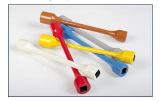
Sockets can be made in a variety of special materials. Stainless steel, bronze, beryllium copper, plastic, and titanium are some of special material used.
