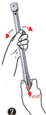
Rotate the locking ring to adjust the torque by the other hand
